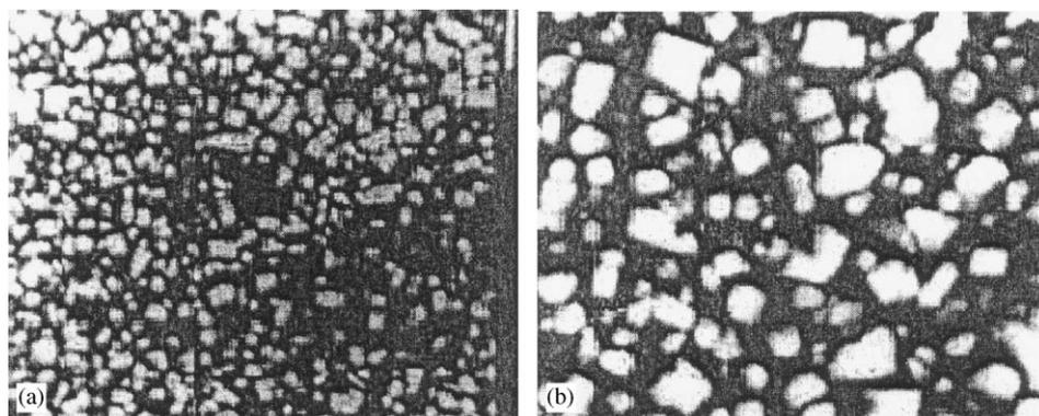
Fig. 4. Scanning electron micrographs of typical Cu<sub>2</sub>O films (a) as-deposited, (b) annealed at 350 °C in air.
