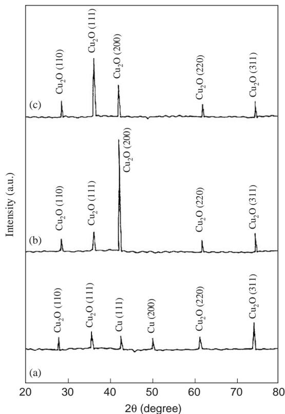
Fig. 1. XRD patterns of  $\text{Cu}_2\text{O}$  films deposited at various solution pH values. (a) pH:  $7.0 \pm 0.1$  (b) pH:  $9.0 \pm 0.1$  (c)  $11.0 \pm 0.1$ ; deposition potential:  $-0.555 \text{ V}$  vs SCE, bath temperature :  $70^\circ \text{C}$ , deposition time: 30 min.
