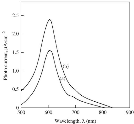
Fig. 5. Variation of photocurrent with wavelength for p-Cu<sub>2</sub>O solar cell (a) as-deposited, (b) annealed at 350 °C in air.
